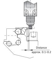
After installation, it is necessary to fully test the functionality of the mechanical limit switch.
