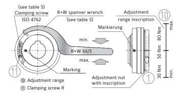
R+W torque limiters are preset and marked with the desired disengagement torque setting at the factory. The min. and max. of the torque adjustment range (10) are also marked on the adjustment nut (1). The disengagement torque is continuously adjustable within the prest range (10) by turning the adjustment nut, increasing or descreasing the tension on the disc springs (2).
