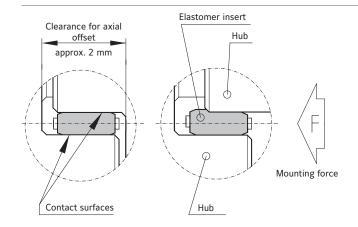
The elastomer insert is the compensating element in an SLE coupling. It transmits torque without backlash and damps shock and vibration. The SLE coupling's elastomer insert determines the hysteresis characteristics of the entire rotational axis, and is available in two different designs.
