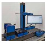
tion process at R+W. All couplings as well as their individual components are inspected by the QA department before they are delivered to customers. A contourograph is now enabling the QA team
